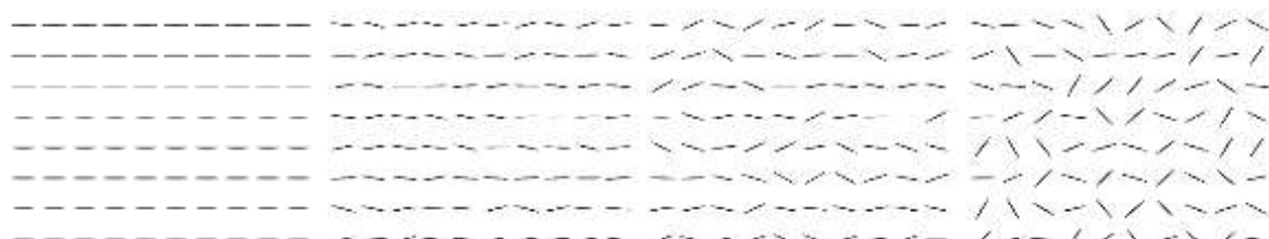
Fig. 1. The distortion of the regular structure of the particles. The particles are represented by uniform discs with 20 px diameter. The distance between the center of the discs is 50 px in (a) image. The position of the discs is randomized within a range of \pm 5 px (b), \pm 10 px (c), and \pm 20 px (d).
