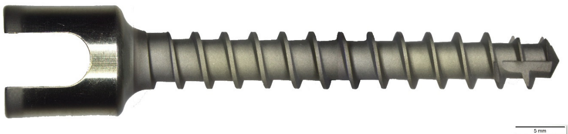
Fig. 1. The designed and grit blasted implant
