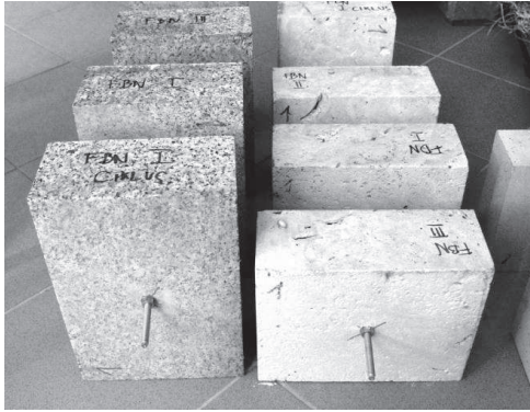
Figure 6. Granite and limestone blocks for pull-out tests.
