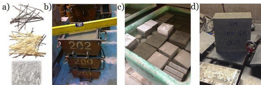
Fig. 1. (a) Fibers: Steel, Plastic, Glass; (b) Cradling; (c) Storage in water; (d) Demoulding of concrete
