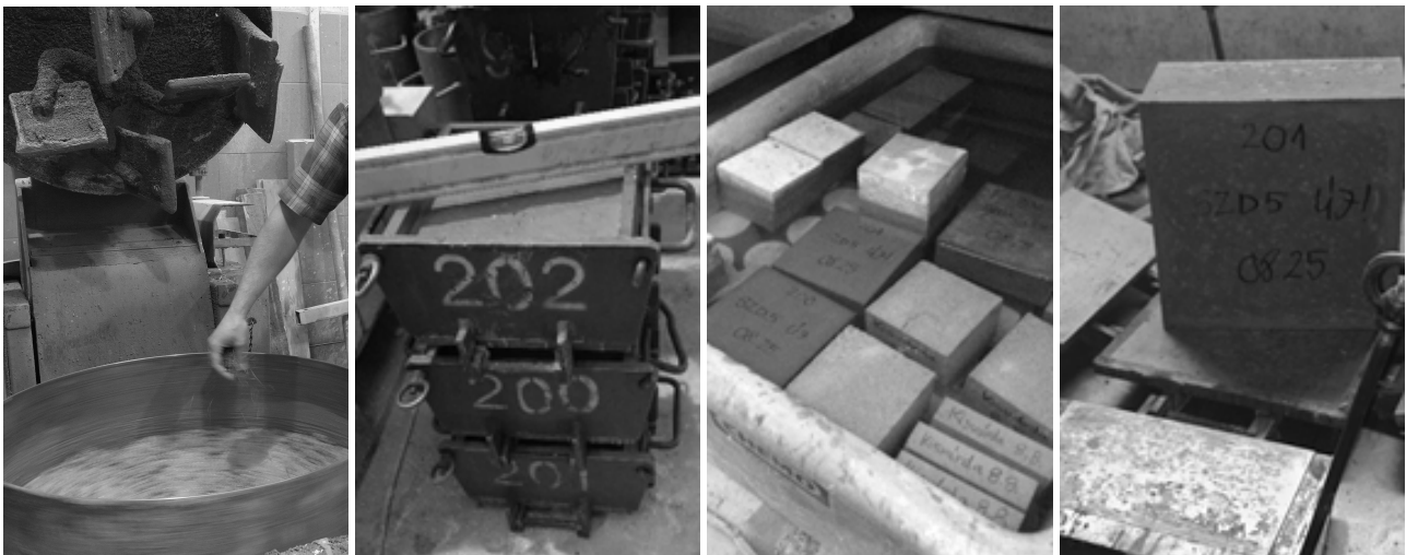
Fig. 1. Mixing and fiber addition; Cradling; Aftercare; Demoulding
