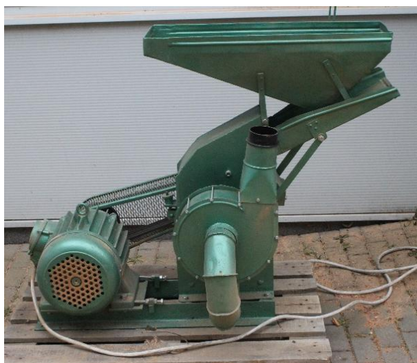
Figure 2. The hammer mill used for fibre production
