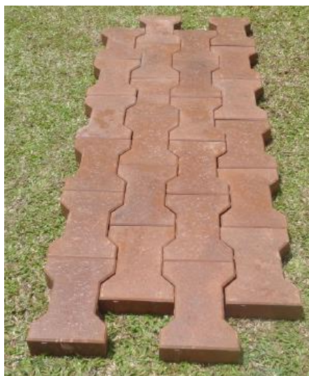
Figure 2. Paving blocks made out of geopolymerised fly ash and red mud mixtures [28]
