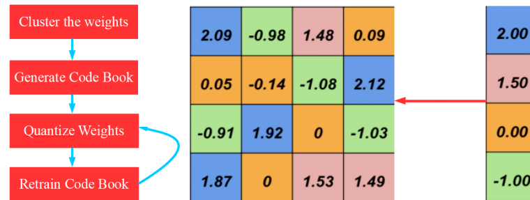
Figure 10.12: Weight sharing (left) and the scheme of weight quantization (right).
