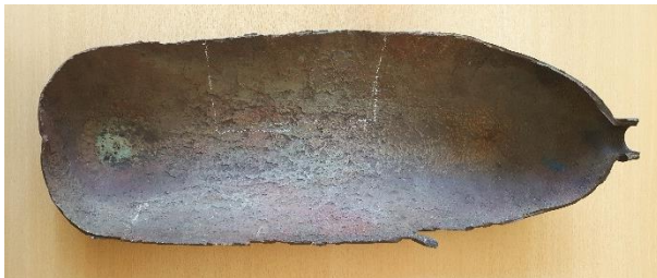
Fig. 1. Severely corroded collapsed structure of scuba diver's tank.
