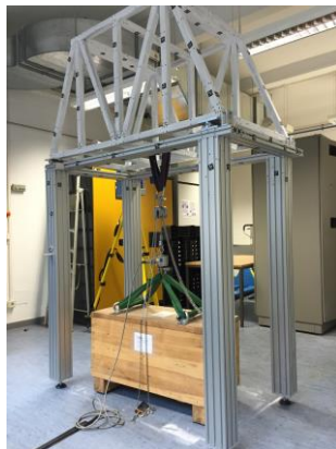
Fig. 1. The bridge specimen on the pedestal, approximately 2147.6 N was applied
