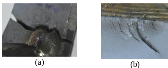
Fig. 5. Visualization of the crack in the upper beam: (a) bottom view; (b) fatigue fringes.
