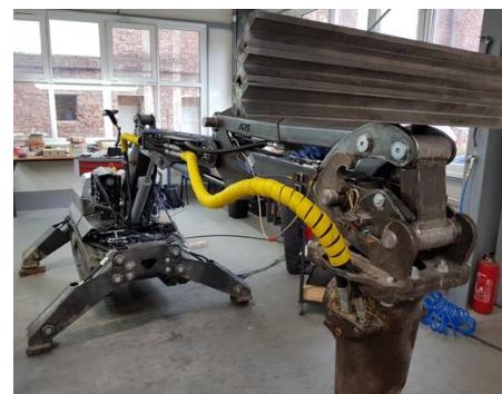
Fig. 3. Example of the load of the robot's arm system – steel beams with a total weight \approx 48 kg
