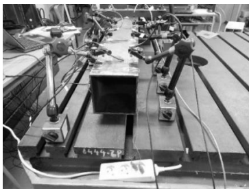
Fig. 4. Measurement of temperatures and deformations under thermal loading.
