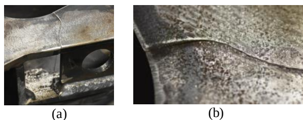
Fig. 4. Visualization of the crack in the frame's arm (a) general view; (b) magnified view of the upper part.
