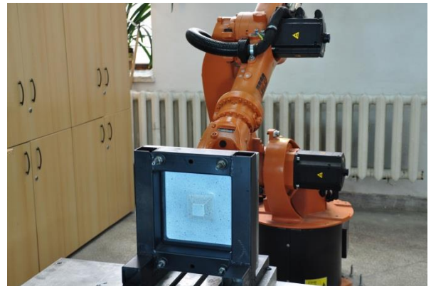
Fig. 1. Experimental layout for researches on single point incremental forming process
