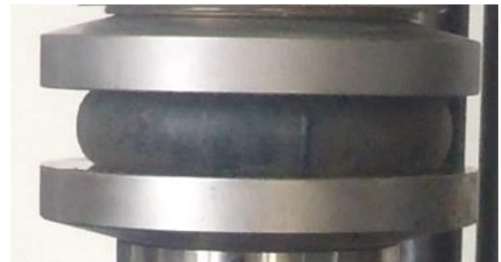
Fig. 2. Deformation of the cylindrical bumper at maximal deflection.
