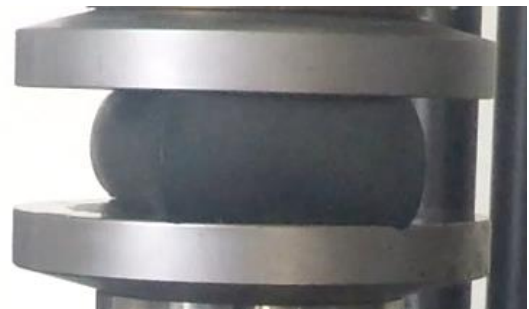
Fig. 3. Deformation of the trapezoidal bumper at maximal deflection.
