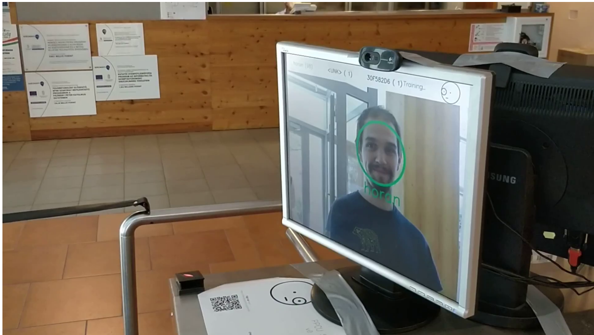
Figure 2.5: Photo of user interface of the Edge. On the screen, one can see the video stream recorded by the camera, but detected faces are circled, and by the top of the screen list of most probable predictions are listed as well as the strength of prediction.
