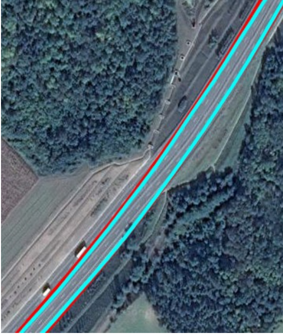
Fig. 11. Smartphone GPS compared to DGPS signal
