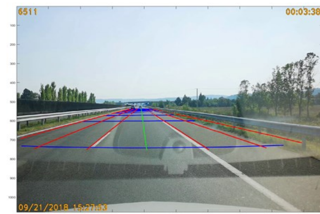
Fig. 5. The result of the homography
