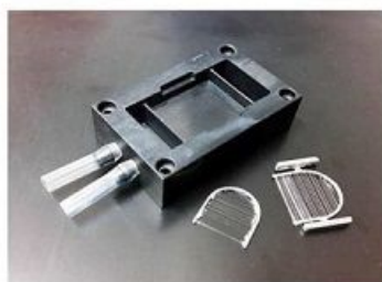
Fig. 2: The components of complete slice chamber
