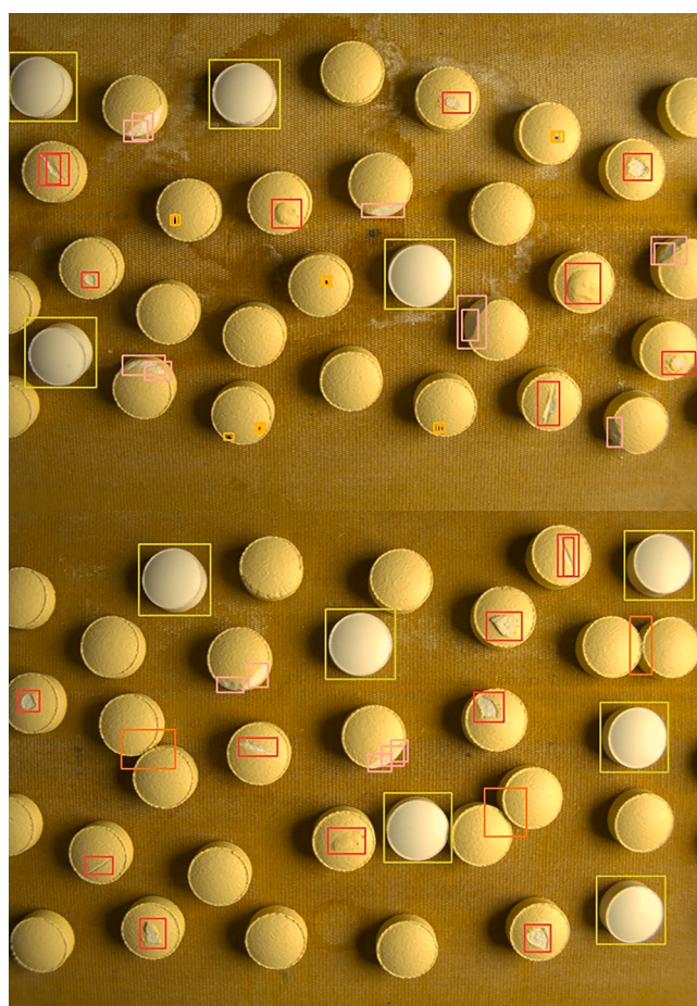
Fig. 4. Two images with classified tablets. Bounding box colouring: yellow: uncoated tablet; light orange: dotted defect; dark orange: twinning tablets; red: uneven surface; pink: edge defect. (For interpretation of the references to color in this figure legend, the reader is referred to the web version of this article.)
