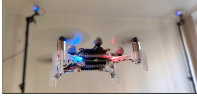
Fig. 6. Experimental setup: OptiTrack Prime 13 infrared cameras and a Crazyflie 2.1 quadcopter with reflective markers.
