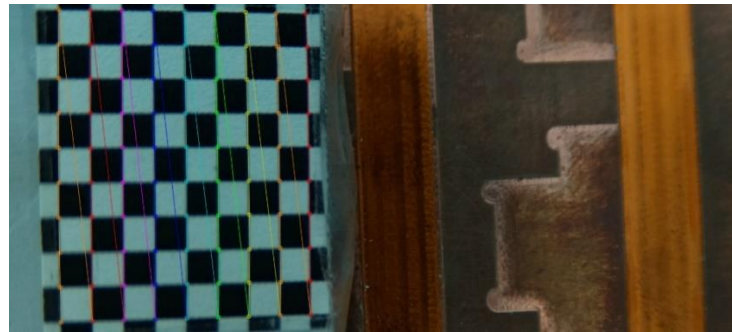
Figure 19: Distortion calibration using a chessboard pattern
