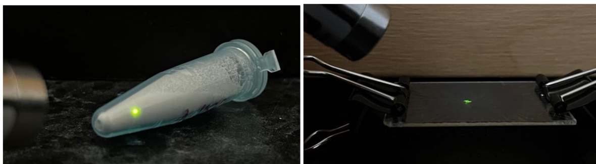
Figure 38. Samples irradiated by 980 nm NIR laser light source ( P < 50 mW): Er-doped UCNPs-powder (left) and chitosan matrix composite coating of Er-doped UCNPs (right)
