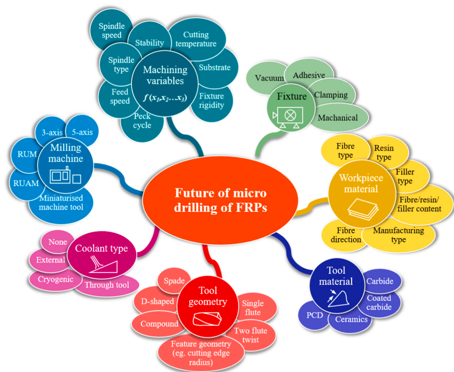
Fig. 19. Variables for exploration and data capture in micro-drilling and mechanical testing.
