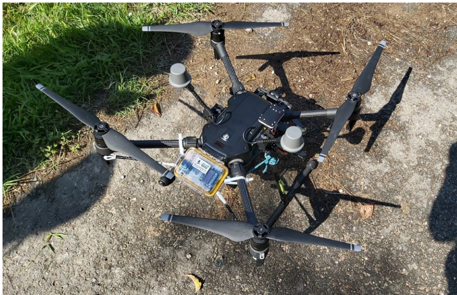
Figure 2. DJI Matrice 210 V2 RTK UAS with the attached Safecast sensor
