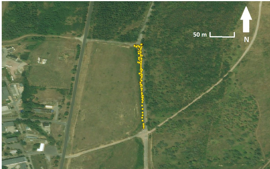
Figure 5. The drone track with the attached Safecast sensor 10 m above the surface
