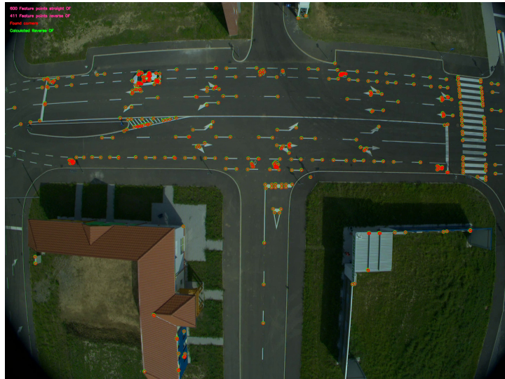
Figure 3.3: Feature points detected by ORB detector.
