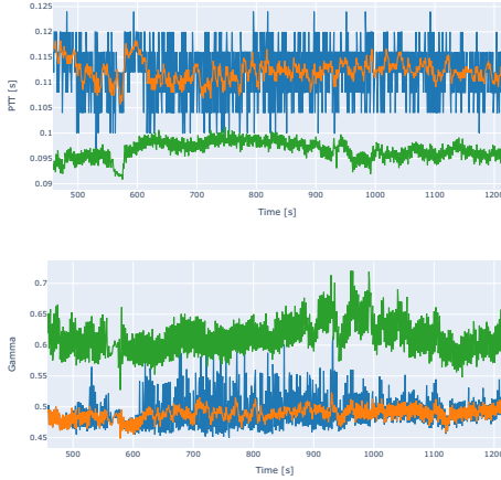
Fig. 4. PTT values calculated directly from the measurements (blue), the curve of the averaged PTTs (orange) using a 7 sample moving window, and the curve of the identified PTT values (green) and the corresponding \Gamma parameters
