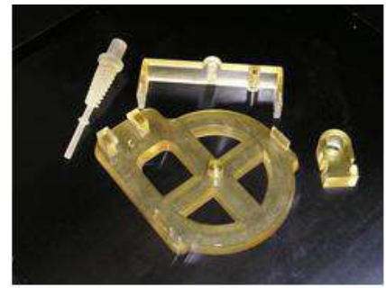
Figure 2. Three stages of additive manufacturing by Objet Eden 350V machine: preparing geometry in electronic format (STL) and importing it into the slicing software, manufacturing, models printed after cleaning
