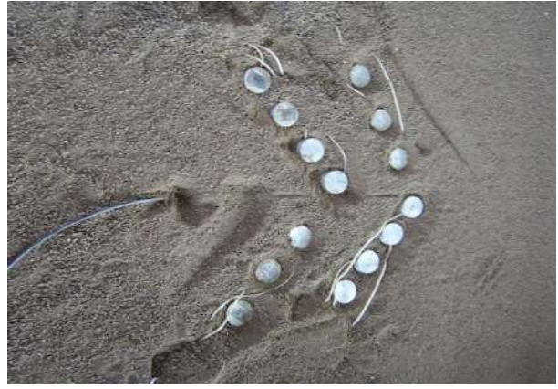
Figure 7. Placement of sensors under the tyre
