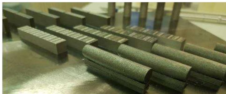
Figure 6. Cuboid and cylindrical test specimens produced by the SLM machine in horizontal and vertical orientation
