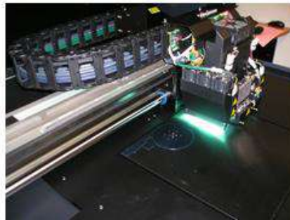
Figure 2. Three stages of additive manufacturing by Objet Eden 350V machine: preparing geometry in electronic format (STL) and importing it into the slicing software, manufacturing, models printed after cleaning
