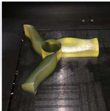
Figure 3. Additive manufacturing of the rotor of a small scale wind generator: body model, printed part on the tray at the end of manufacturing still surrounded by support material, after cleaning
