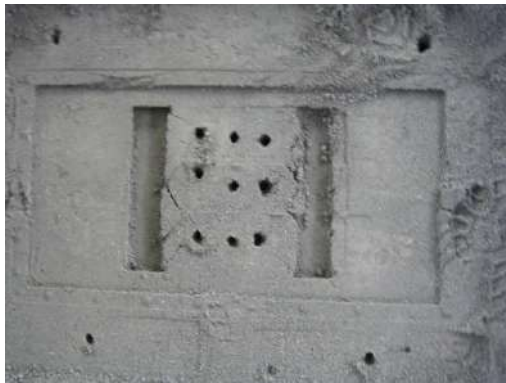
Figure 6. The penetrometer test points and initial and post-load values at different depths
