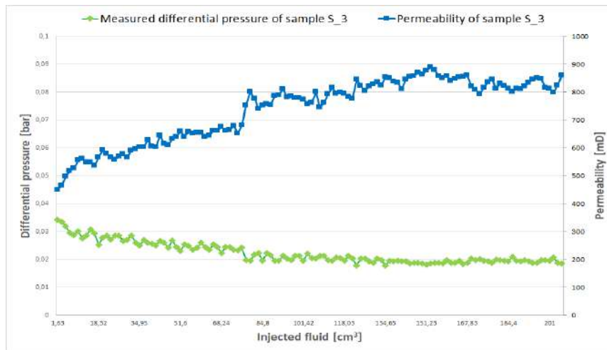
Figure 4 The measured differential pressure and permeability of sample S-3
