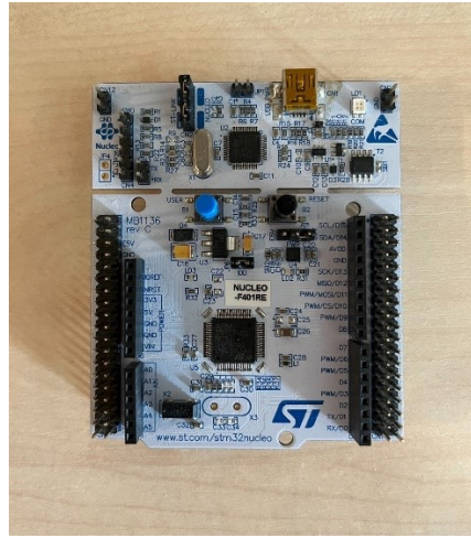
Figure 13. The STM32 F401RE microcontroller used to implement our proposed model-driven classifier.
