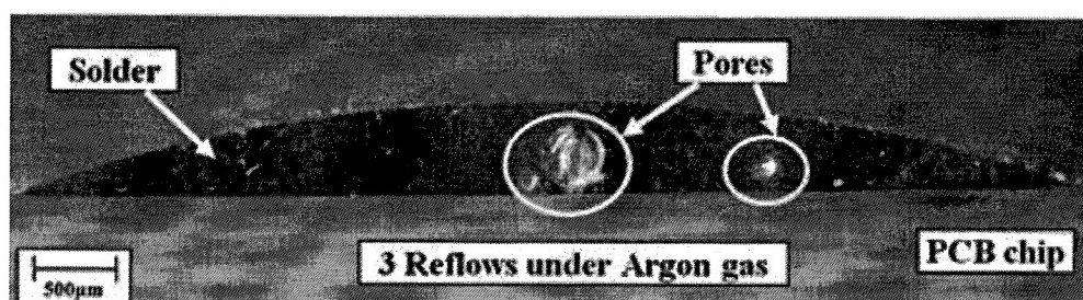
Fig. 5. Pores in the cross section of solder (full colour version available online)
