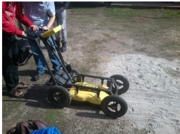
GPR survey in progress
