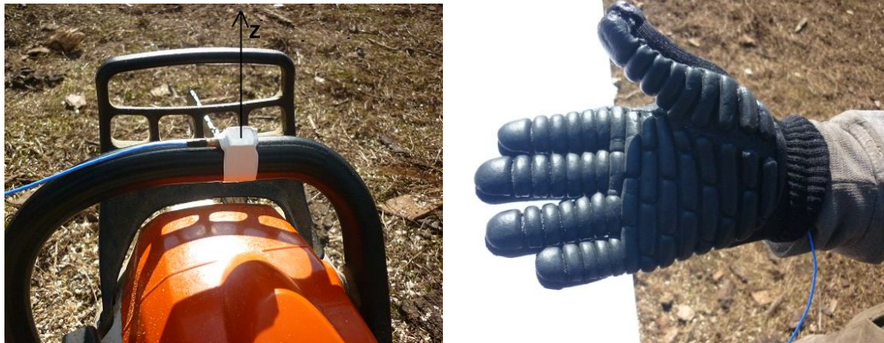
Figure 6. Measurement point on the chainsaw (left) and Portwest A 790 anti-vibration glove (right)
