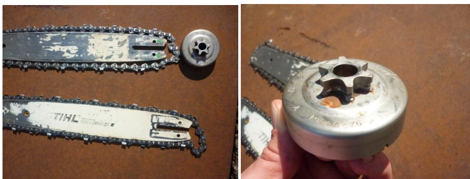
Figure 5. New and weared chains and chain-wheels
