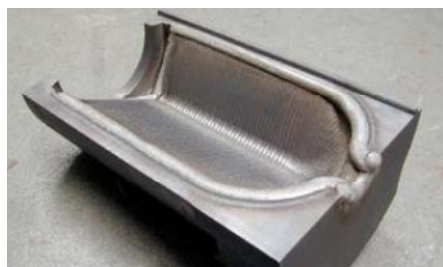
Figure 7. PTA welded mould
